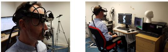
(a) Eye-Link II Headset (b) Complete Apparatus
